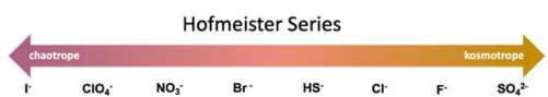
Fig. 3 Common reference anions in the Hofmeister series. This represents a common reference framework for electrochemical sensors. Electrochemical sensors are commonly more sensitive to charge diffuse chaotropes (left) than charge dense kosmotropes (right). In this study, we place \text{HS}^- in the series between \text{Cl}^- and \text{Br}^- ( vide infra ).
