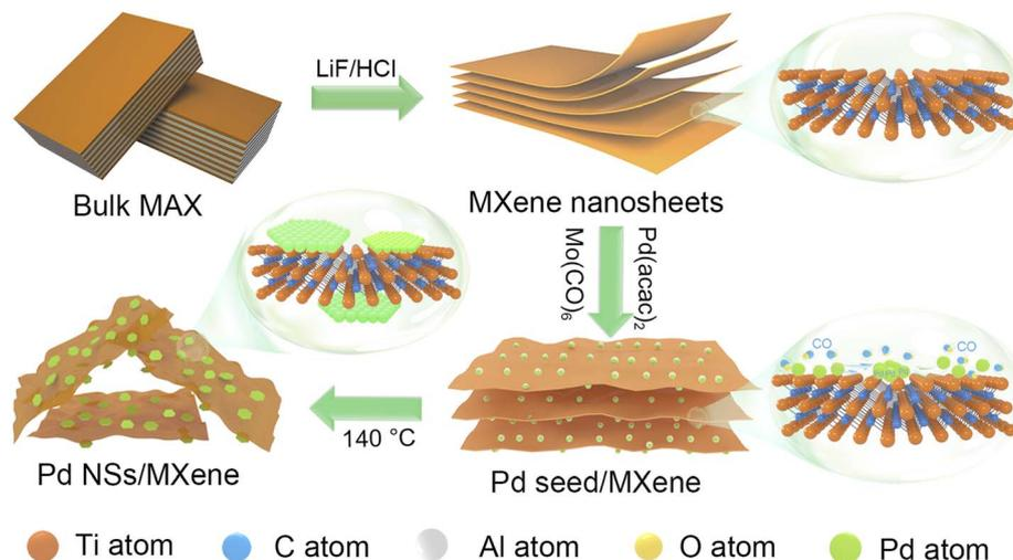
**Fig. 1** The synthesis process of the 2D/2D Pd NSs/MXene heterojunction: (1) synthesis of 2D MXene nanolayers by a LiF and HCl etching route; (2) growth of Pd seeds on the surface of MXene as well as the generation of CO molecules by the decomposition of  $\text{Mo}(\text{CO})_6$ ; (3) gradual formation of 2D Pd nanosheets on the MXene nanosheets.
