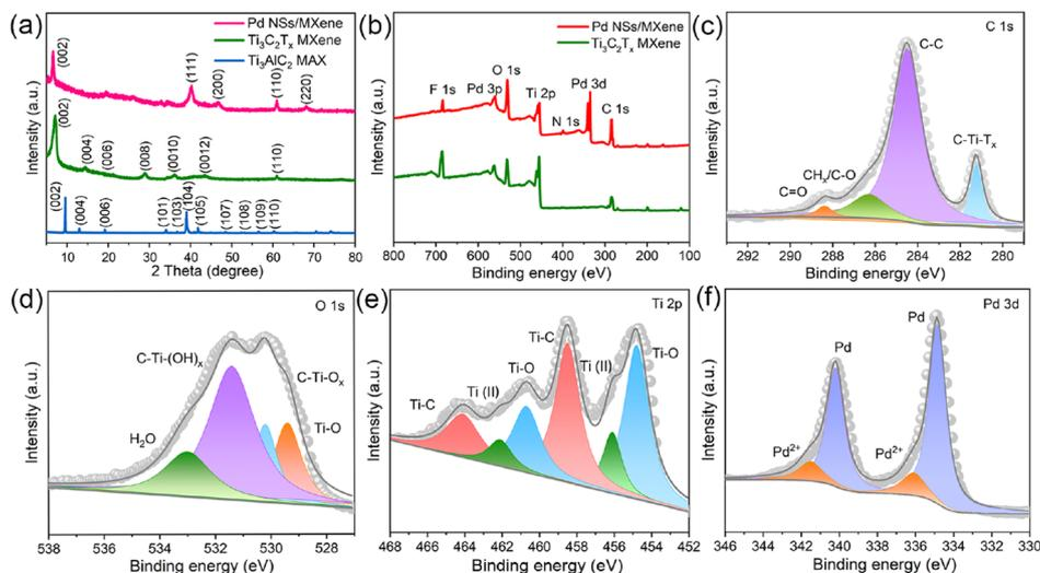
**Fig. 3** Structural characterization of the Pd NSs/MXene heterojunction. (a) XRD patterns of the Pd NSs/MXene,  $\text{Ti}_3\text{C}_2\text{T}_x$  MXene, and  $\text{Ti}_3\text{AlC}_2$  MAX samples. (b) XPS survey spectra of Pd NSs/MXene and  $\text{Ti}_3\text{C}_2\text{T}_x$  MXene. The typical (c) C 1s, (d) O 1s, (e) Ti 2p, and (f) Pd 3d core-level XPS spectra of Pd NSs/MXene.
