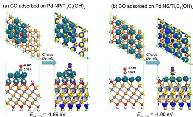
Fig. 7 The relaxed atomic structures for the adsorption of a CO molecule on the (a) Pd NP/ $\text{Ti}_3\text{C}_2(\text{OH})_x$  and (b) Pd NS/ $\text{Ti}_3\text{C}_2(\text{OH})_x$  models as well as the corresponding deformation charge density near the CO molecule. The blue and yellow colors indicate the charge increase and depletion of electrons, respectively.
