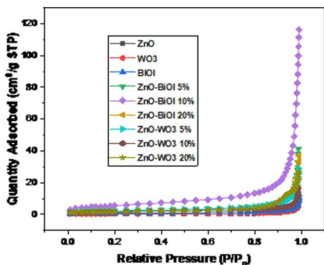
Fig. 3 N<sub>2</sub> adsorption-desorption isotherms of the as-prepared bare catalysts and heterostructures.
