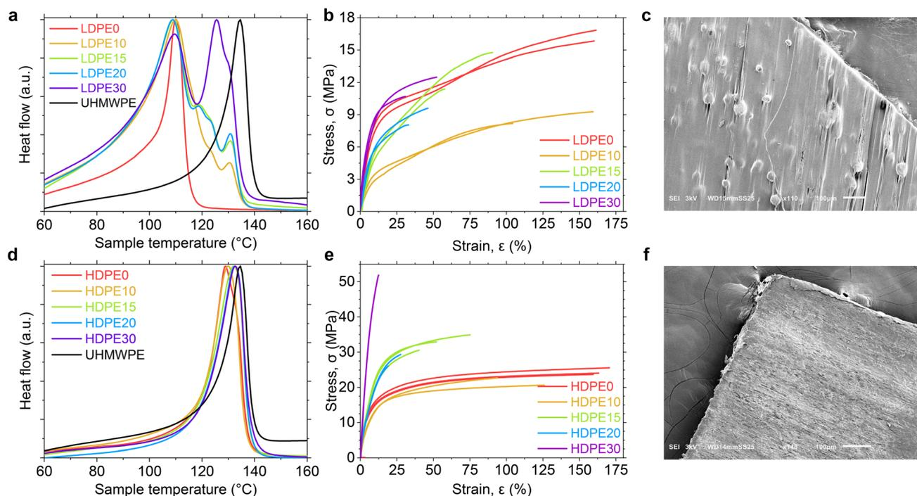
**Fig. 5** (a and d) DSC thermograms (20 K min<sup>-1</sup>, second heat), (b and e) engineering stress–strain curves (DMA force ramp) of LDPE/UHMWPE and HDPE/UHMWPE microcompounded blends across a composition range of 0–30 wt% UHMWPE; SEM images of LDPE/UHMWPE (c) and HDPE/UHMWPE (f) at 15 wt% UHMWPE.
