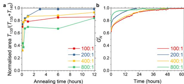
**Fig. 2** (a) Normalised area  $T_{135^{\circ}\text{C}}/(T_{135^{\circ}\text{C}} + T_{140^{\circ}\text{C}})$  as a function of annealing time, and (b) normalised storage modulus ( $G'_{\text{N}}$ , measured at  $160^{\circ}\text{C}$ ,  $\omega = 10 \text{ rad s}^{-1}$ ) as a function of time of polyethylene synthesised by  $1_{\text{sMAO}}$  of varying  $[\text{Al}_{\text{sMAO}}]/[\text{Ti}]$ .
