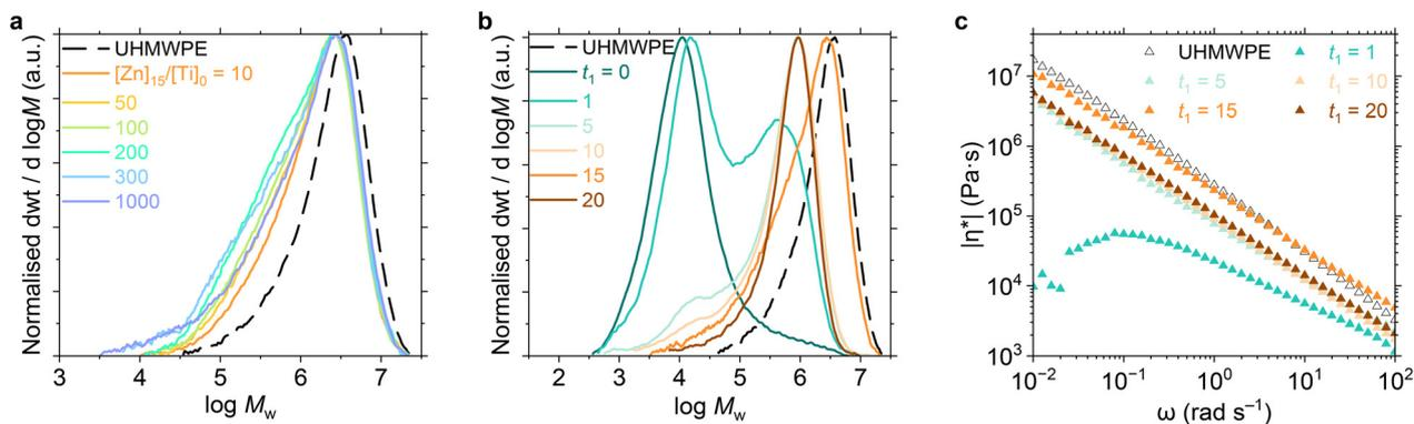
**Fig. 3** (a and b) Gel-permeation chromatograms, and (c) rheological complex viscosity (SAOS frequency sweep measured at 160 °C) of polyethylene as a function of  $[Zn]_{t_1}/[Ti]_0$  for polymerisation in the presence of  $ZnEt_2$  ((a)  $t_1 = 15$  minutes; (b and c)  $[Zn]_{t_1}/[Ti]_0 = 1000$ ).
