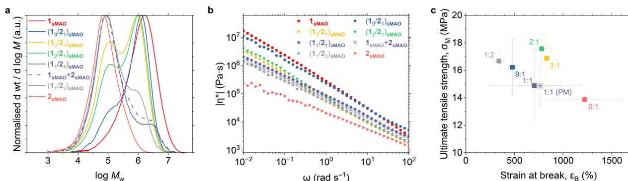
Fig. 4 (a) Gel-permeation chromatograms; (b) rheological complex viscosity (SAOS frequency sweep measured at 160 °C); (c) tensile results of polyethylene produced at  $T_p = 60$  °C by coimmobilised multisite catalysts  $(1_n/2_m)_{\text{sMAO}}$  (or the physical mixture  $1_{\text{sMAO}} + 2_{\text{sMAO}}$ ) as a function of  $[\text{Ti}]/[\text{Zr}]$ .
