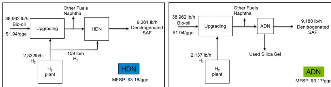
Fig. 7 Comparison of the impacts on the MFSP from the different denitrogenation methods in the process of converting wet waste to SAF and other fuels using HTL technology.
