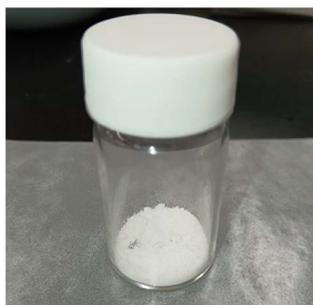
Fig. 9 A photograph of the Mg[TFSA]<sub>2</sub> sample after NH<sub>3</sub> absorption/desorption cycles at 300 K. Mg[TFSA]<sub>2</sub> sample in the glass bottle ( $\varnothing$  24 mm, 10 mL).
