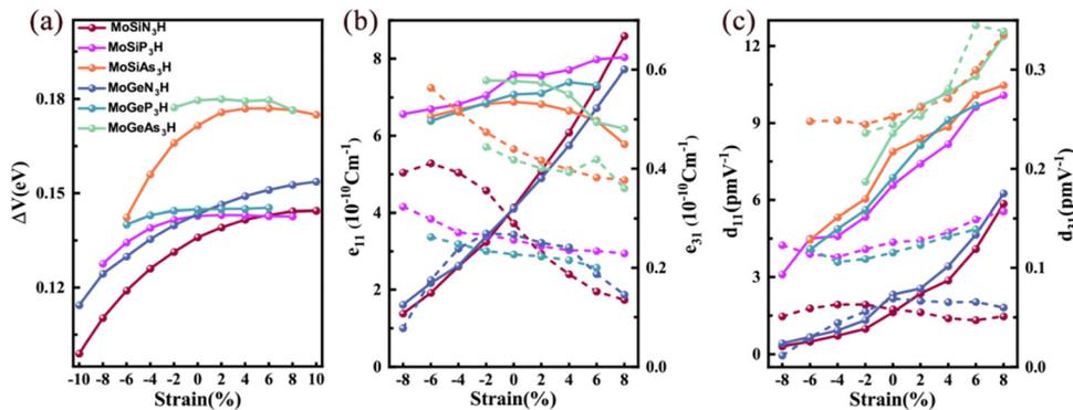
Fig. 7 (a) Spin-valley coupling at the  $K$  point, (b) piezoelectric coefficients  $e_{11}/e_{31}$  and (c)  $d_{11}/d_{31}$  under biaxial strain in the MoAZ<sub>3</sub>H MLs. In the three panels, the solid lines in one color and the corresponding dashed lines indicate the results of the same material.
