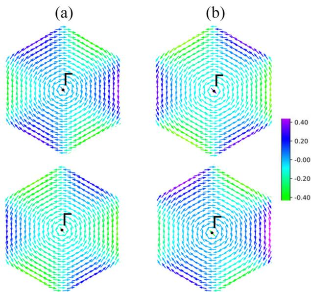
Fig. 4 Spin texture for the two highest spin-split valence bands in (a) MoSiP<sub>3</sub>H and (b) MoGeAs<sub>3</sub>H MLs calculated in the entire BZ, where (a) and (b) include the upper and lower valence bands, respectively. Here, the arrows show the in-plane components of spin polarization, and the colors represent the out-of-plane components of spin polarization.
