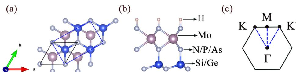
Fig. 1 (a) and (b) are the top and side views of the crystal structures, and (c) the high symmetry path in the Brillouin zone for the  $\text{MoAZ}_3\text{H}$  MLs, respectively. In panel (a), black rhombi and blue rectangles represent the unit cells and rectangular supercells of the  $\text{MoAZ}_3\text{H}$  MLs, respectively.
