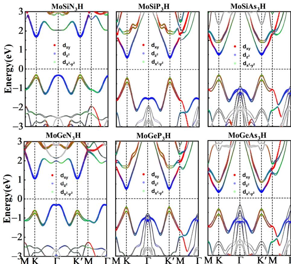
Fig. 2 Orbital-resolved band structures of the d-orbitals of Mo atoms in MoAZ<sub>3</sub>H MLs.
