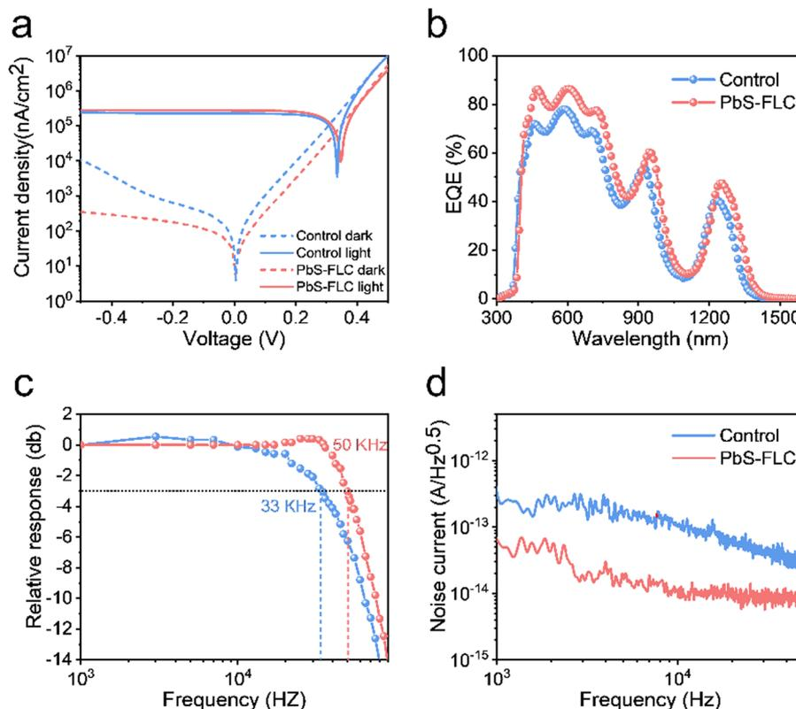
Fig. 5 (a)  $J$ - $V$  curves of the FLC and control devices measured under dark conditions and  $1300 \text{ nm}$  light illumination. (b) EQE curves of the  $1250 \text{ nm}$  PbS CQD devices. (c)  $-3 \text{ dB}$  bandwidth. (d) Noise power spectra of the control and FLC devices.
