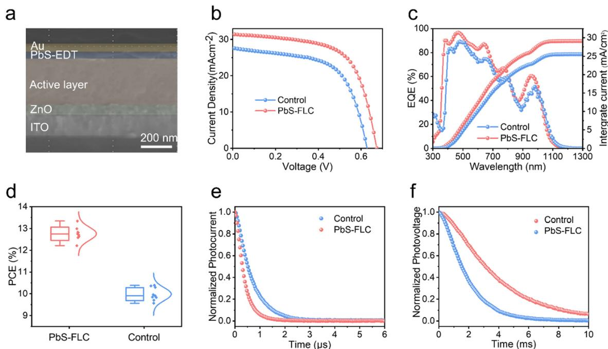
Fig. 4 (a) Cross-sectional SEM image of the device architecture. (b)  $J$ - $V$  curves of FLC and control devices. (c) External quantum efficiency (EQE) curves and integrated  $J_{sc}$  of the 940 nm PbS CQD solar cells. (d) Distribution of PCE values. Transient photocurrent (e) and photovoltage (f) decay spectroscopy of the FLC and control devices.
