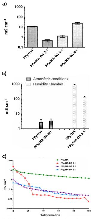
**Fig. 13** (a) Conductivities of PPy/HA and PPy/(HA–DA) films on a poly(dimethylsiloxane) substrate. (b) Conductivities of PPy/HA and PPy/(HA–DA) 8:1 films under different humidity conditions. (c) Conductivity as a function of applied stress; conductivity measurements are shown as the mean and standard deviation of n = 3. Reproduced, with adaptations, from ref. 233 with permission from Elsevier; copyright © 2017 Elsevier B.V.
