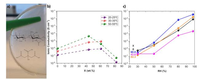
**Fig. 28** (a) Section of the prepared CSA/citric acid film, with the structures of both the GAG and the organic acid; (b) ionic conductivity isotherms obtained at RH < 30%; and (c) relative humidity dependence of the ionic conductivity under different RH at 25 °C for CSA and CA:CSA(X), with different w/w ratios (X = 0, 43.6, 60.8 and 82.3). Reproduced from ref. 47 with permission from Elsevier; copyright © 2019 Elsevier Ltd.
