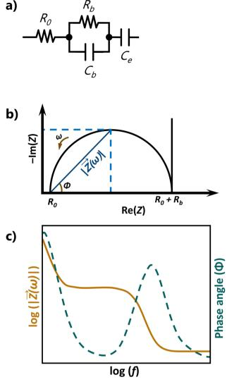
Fig. 9 (a) Equivalent circuit, (b) Nyquist plot, and (c) Bode plot for an ideal ion conducting electrolyte.
