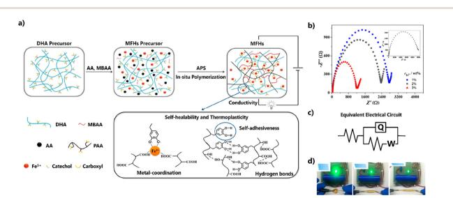
Fig. 19 (a) Schematic of the synthetic process for the multifunctional conductive hydrogels and the corresponding interactions inside multifunctional networks; (b) electrochemical impedance plot of the hydrogels with different  $c(Fe^{3+})$ , and (c) the corresponding equivalent electrical circuit; and (d) images of strain-dependent conductivity performance of the hydrogels. Reproduced from ref. 436 with permission from The American Chemical Society. Copyright © 2019.
