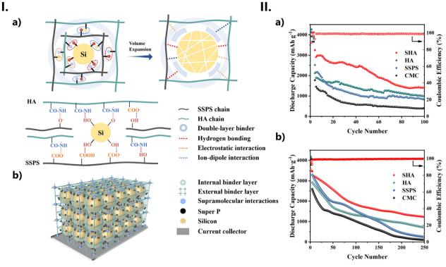
**Fig. 22** (I) (a) Schematic diagram of the double-layer binder network resisting against volume expansion and illustration of supramolecular interactions between HA and Si NPs. (b) 3D network of Si anodes with HA as binder. (II) Cycling performance of various binders at (a) 4 A  $g^{-1}$  and (b) 2 A  $g^{-1}$ . Reproduced from ref. 222 with permission from Elsevier; copyright  $\bigcirc$  2018 Elsevier B.V.
