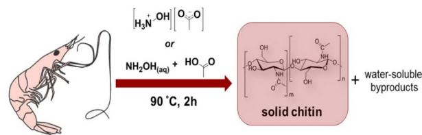
Fig. 14 Scheme of the extraction of chitin from “biowaste” feedstock. Reproduced from ref. 166 with permission from American Chemical Society, copyright 2016.
