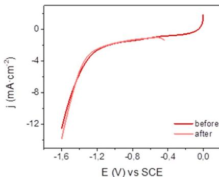
Fig. 7 Linear sweep voltammetry of Mn@Terpy-COF|NT ([Mn]<sub>total</sub> = 850  $\mu\text{mol cm}^{-2}$ ) on CP at 10  $\text{mV s}^{-1}$  before and after CPE at  $-1.3$  V vs. SCE in water  $\text{K}_2\text{SO}_4/\text{K}_2\text{B}_4\text{O}_7$  under  $\text{CO}_2$ .
