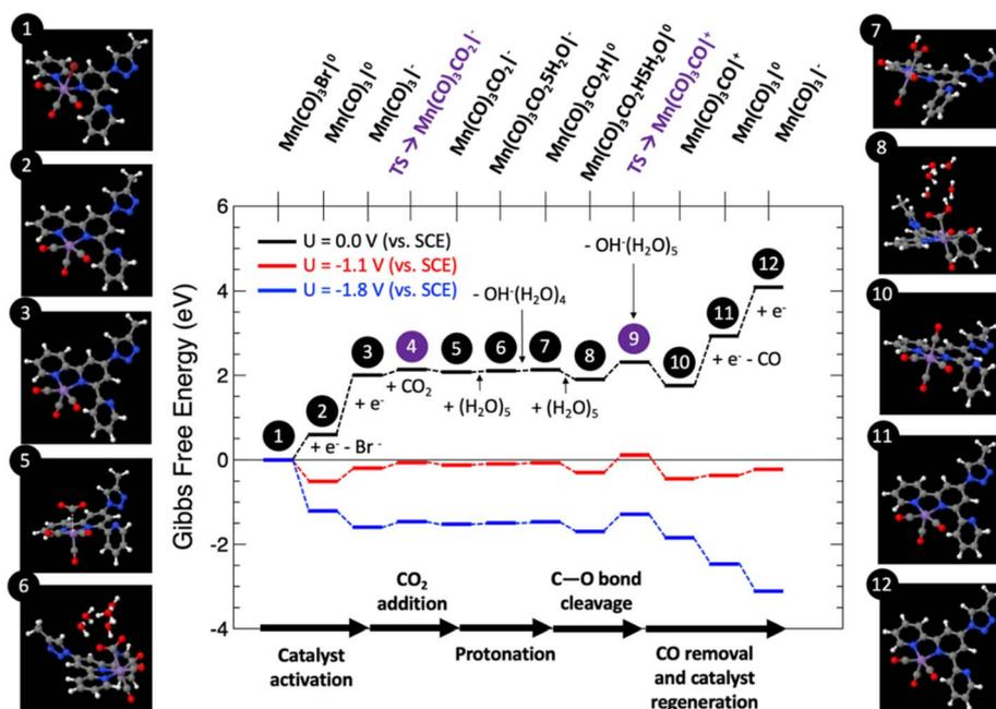
Fig. 9 Computed Gibbs free energy diagram (in eV) for the CO<sub>2</sub>RR towards CO evolution at different applied voltages of  $U = 0$  (black path),  $-1.1$  (red path) and  $-1.8$  V (blue path) *vs.* SCE. Calculated geometries of all the intermediates are shown numbered according to the reaction path steps, indicating each sub-reaction of the mechanistic path.
