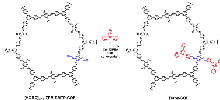
Scheme 1 Synthesis of Terpy-COF from  $[\text{HC}\equiv\text{C}]_{0.17}\text{-TPB-DMTP-COF}$ .
