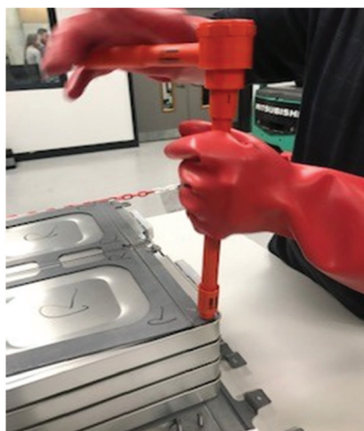
Fig. 5 (a) Pouch cell tabs ultrasonically welded to copper busbar, (b) module interconnections utilising threaded bolts through solid busbars (c) dismantling of pack sub-assemblies using standard shop tooling – all Nissan Leaf 1 st generation.
