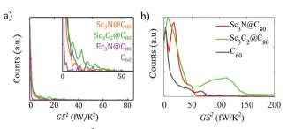
**Fig. 6** Power factor  $GS^2$  analysis. a) Experimental 1D histograms of power factor at first contact, built with the data in Fig. 3. The inset zooms into the details of the main panel. b). Theoretical 1D histograms of power factor obtained from Fig. S46 of the ESI.†
