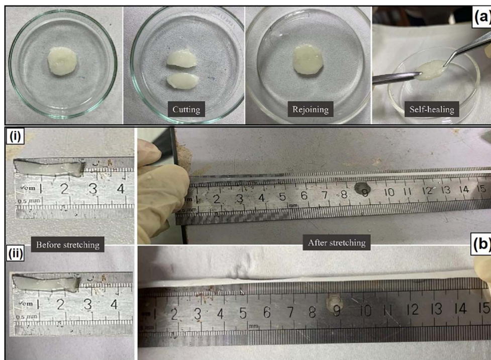
Fig. 13 (a) Digital images of the S48 hydrogel sample. After cutting into two pieces and pressing together for a duration of 30 minutes at 60 °C, it merges into a single piece and (b) photograph of hydrogels before and after stretching exercise for (i) S48 and (ii) S72. Reproduced with permission from ref. 47 Copyright (2023), Elsevier Inc.
