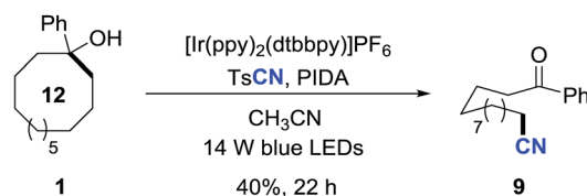
B. Ring-opening alkynylation of large-sized cycloalkanol
