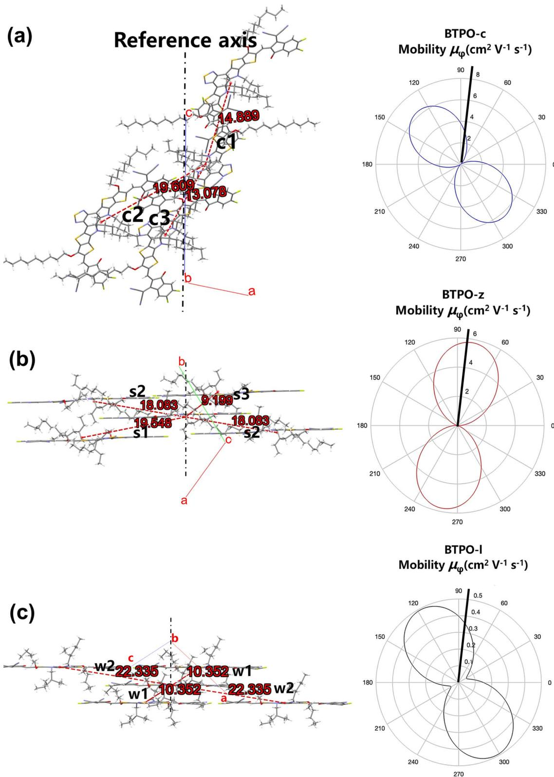
Fig. 8 (a–c) Molecular packing viewed along the normal to the plane of interest (left: the number in green stands for the hopping distance ( $r$ , Å)) and corresponding simulated anisotropic electron mobility curves based on the hopping model (right) of (a) BTPO-c, (b) BTPO-z and (c) BTPO-l.
