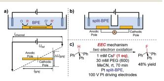
Fig. 24 (a) Schematic of a bipolar electrochemical set-up, demonstrating the formation of anodic and cathodic poles on a bipolar electrode (BPE). (b) Schematic of a split-bipolar electrode in a U-type cell. (c) Fluorination of triphenylmethane can occur at low concentrations of electrolyte solution utilising a BPE set-up, reported by Inagi and co-workers [ref. 83; poly(ethylene glycol) (PEG) additive required to solubilise CsF in acetonitrile].
