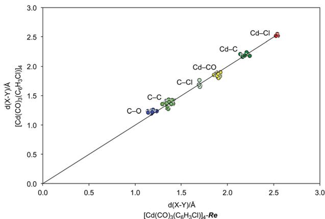
Fig. 7 Comparison of the bond lengths of  $[\text{Re}(\text{CO})_3(\text{C}_4\text{N}_2\text{H}_3\text{S})]_4$ , refined as  $[\text{Cd}(\text{CO})_3(\text{C}_6\text{H}_3\text{Cl})]_4\text{-Re}$ , with those of the published data for  $[\text{Cd}(\text{CO})_3(\text{C}_6\text{H}_3\text{Cl})]_4$ ,<sup>4</sup> demonstrating an excellent correspondence.
