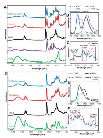
**Fig. 4** ATR-FTIR spectra of CD25 (A–C) and PVA50 (D and E) after curing and after purification compared to HP $\beta$ CD, PVP, PVA and corresponding pPGS spectra. (A and D) Full spectra. (B and E) C=O bands, absorbance normalized to the 1730 cm<sup>-1</sup> band. (C and F) C–O, C–C and C–N bands, absorbance normalized to the 1160 cm<sup>-1</sup> band.
