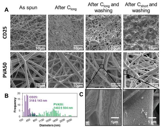
**Fig. 3** Morphology of the fibers as spun and after post-treatments. Low magnification SEM pictures (A), diameter distribution of diameters of as-spun fibers (B) and high magnification pictures of cured PVA50-washed fibers (C). CD25 contains 50% of PGS, 25% of HP $\beta$ CD and 25% of PVP; PVA contains 50% of PGS and 50% of PVA. The morphology is shown here after C<sub>long</sub> (24 h at 120 °C, 48 h at 140 °C and 24 h at 170 °C) and after 24 h washing in water.
