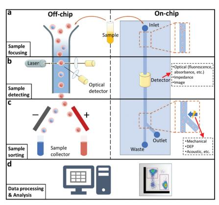
Fig. 1 Schematic illustration of typical off-chip (left side) and on-chip (right side) flow cytometry setup and workflow including (a) Sample focusing. (b) Sample detecting. (c) Sample sorting. (d) Data processing & analysis.
