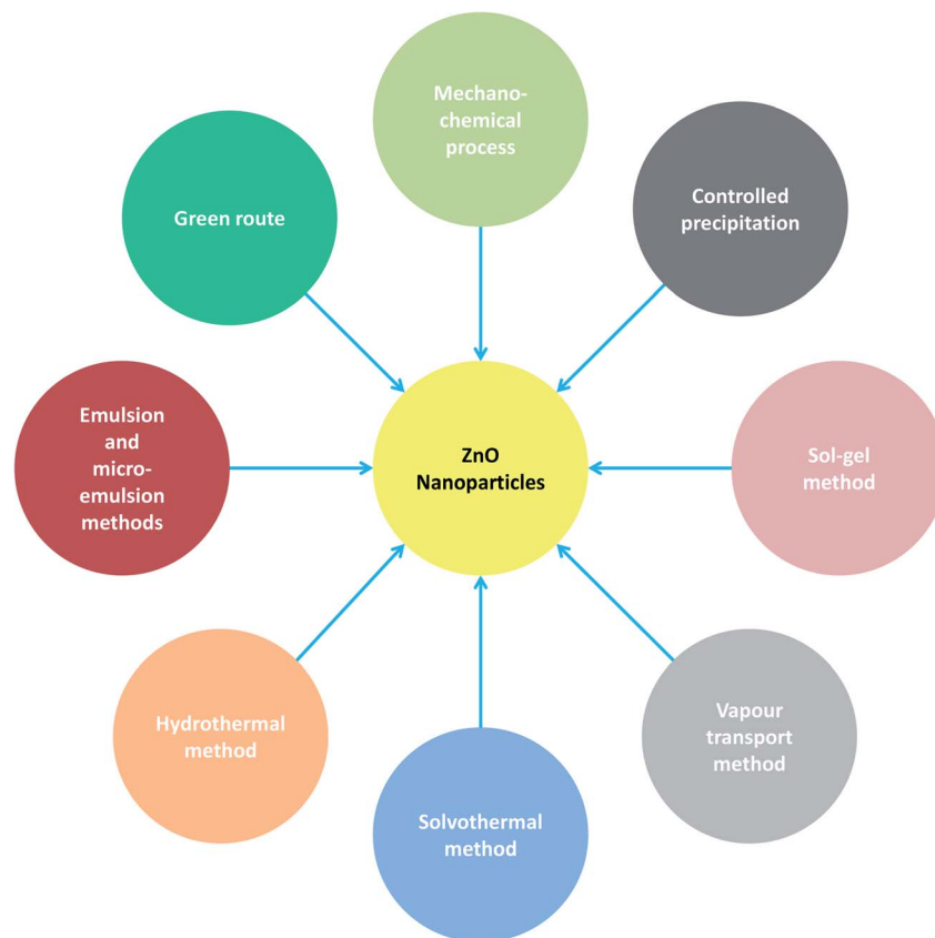
Fig. 1 Various strategies for the fabrication of ZnO NPs.
