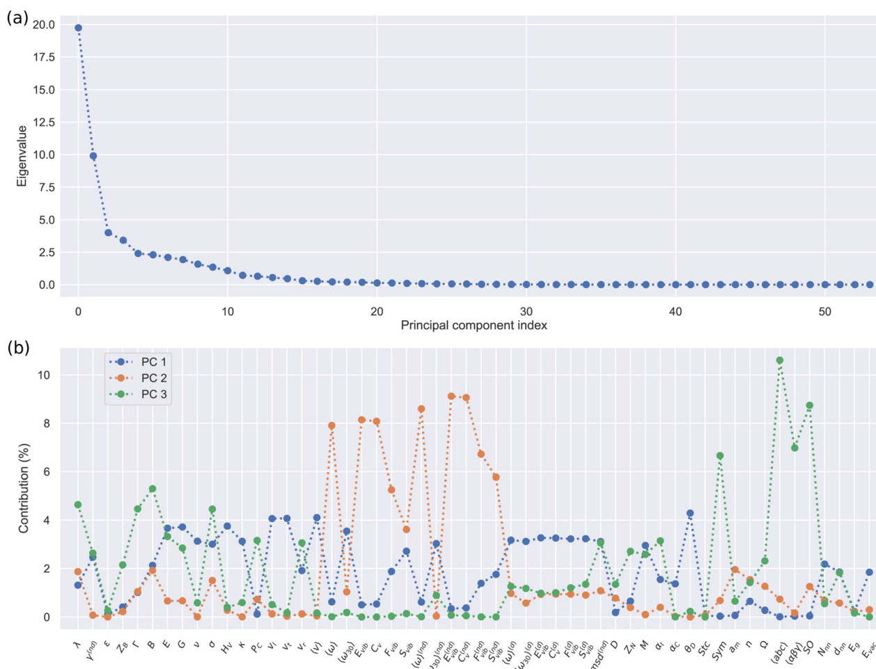
Fig. 4 Principal component analysis results obtained for the SSE DFT-AIMD database. (a) Eigenvalues corresponding to the diagonalization of the Spearman correlation matrix obtained by considering all the materials in the DFT-AIMD database. (b) Eigenvector components of the first three principal components obtained from the diagonalization of the Spearman correlation matrix obtained by considering all the materials in the DFT-AIMD database at T = 500 \pm 100 K.
