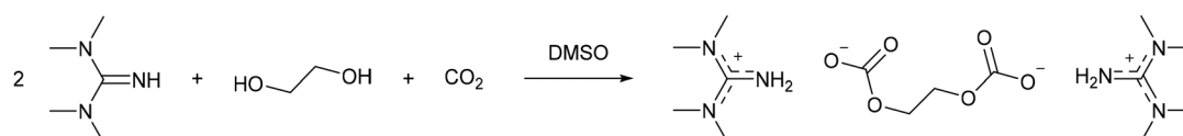
Scheme 4 The formation of a guanidinium ethylene di-carbonate used for non-derivative cellulose dissolution. 41
