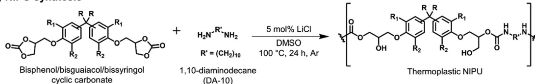
Scheme 1 Synthesis of (a) BGF/BSF using guaiacol/syringol and vanillyl/syringyl alcohol, (b) BGA/BSA using guaiacol/syringol and acetone, (c) diglycidyl ether of bisguaiacol/bisxyringol from respective bisguaiacol/bisxyringol and epichlorohydrin, (d) bisguaiacol/bisxyringol cyclic carbonate from respective diglycidyl ether and \text{CO}_2 , and (e) NIPU using respective bisguaiacol/bisxyringol cyclic carbonate and 1,10-diaminodecane (DA-10).
