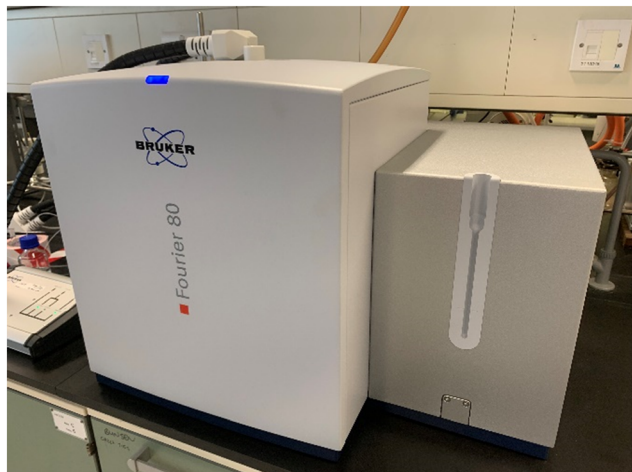
Fig. 5 Image of Bruker 80 MHz benchtop NMR spectrometer.
