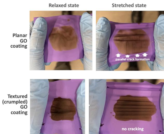
**Fig. 10** Demonstration that compressive pre-texturing of graphene oxide films renders them stretchable, with no cracks observed over multiple stretch and relax cycles. Films (0.5  $\mu\text{m}$  thick) were formed by solution casting of pure graphene oxide (no polymer additive) on nitrile glove cutouts. Still images extracted from video original (see Videos S1 and S2†).
