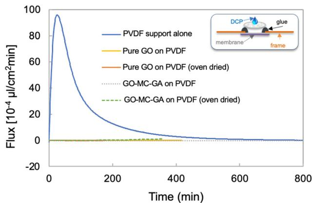
Fig. 6 Diethyl chlorophosphate (DCP) permeation rates through GO (3  $\mu$ m) and GO-MC-GA (10  $\mu$ m) films under conditions of vapor-only contact. All films are supported on a porous PVDF filter during testing, which allows rapid DCP vapor permeation when used alone as a positive control. All films studied here are effective DCP vapor barriers.
