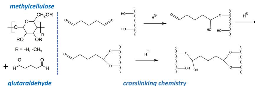
**Fig. 2** Molecular structures and crosslinking mechanism relevant to the GO-MC-GA composite coatings. Glutaraldehyde is reported to be effective as a crosslinker of hydroxyl groups,<sup>45–47</sup> and the mechanism is initiated by nucleophilic attack by hydroxyl oxygen on the carbonyl carbons, resulting in glutaraldehyde fixation to polymer and/or GO by ether linkages.
