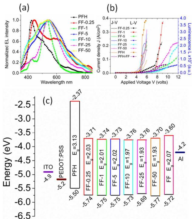
Figure 4. (a) EL spectra of copolymers and PFH (b) Current density-voltage (J-V) and Luminescence - voltage (L-V) plots of OLEDs, (c) Energy level diagram of polymers.
