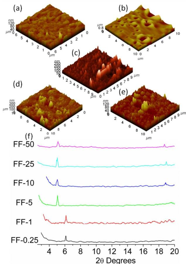
Figure 3. AFM micrograph of (a) FF-0.25, (b) FF-1, (c) PFH-FF, (d) FF-5, (e) FF-10 and (f) GIXRD traces of copolymers.
