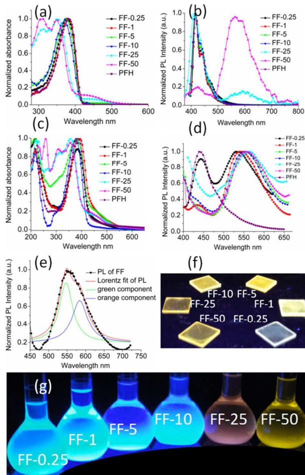
Figure 1. (a) Absorption, (b) PL spectra in THF solution; (c) Absorption, (d) PL spectra in spun thin films of copolymers. (e) Lorentzian fit for PL spectra of FF thin film; (f) spun thin films, (g) THF Solutions of copolymers under irradiation at  $\sim 360$ nm.
