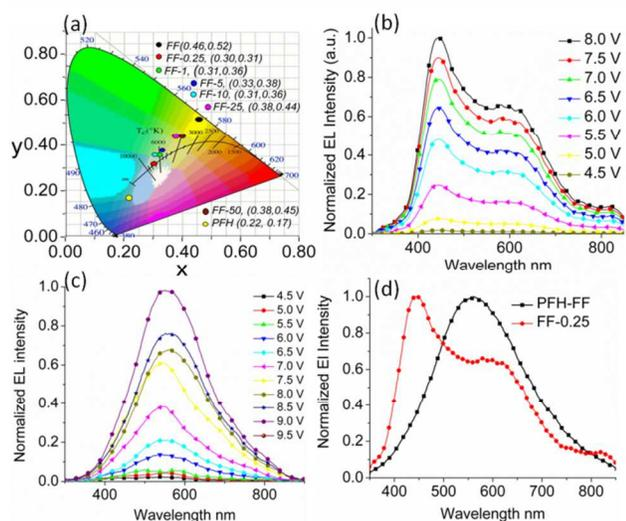
Figure 5. (a) CIE coordinates of polymers; EL spectra of (b) FF-0.25, (c) PFH-FF at different applied voltage and (d) EL spectra of FF-0.25 and PFH-FF at 8V.
