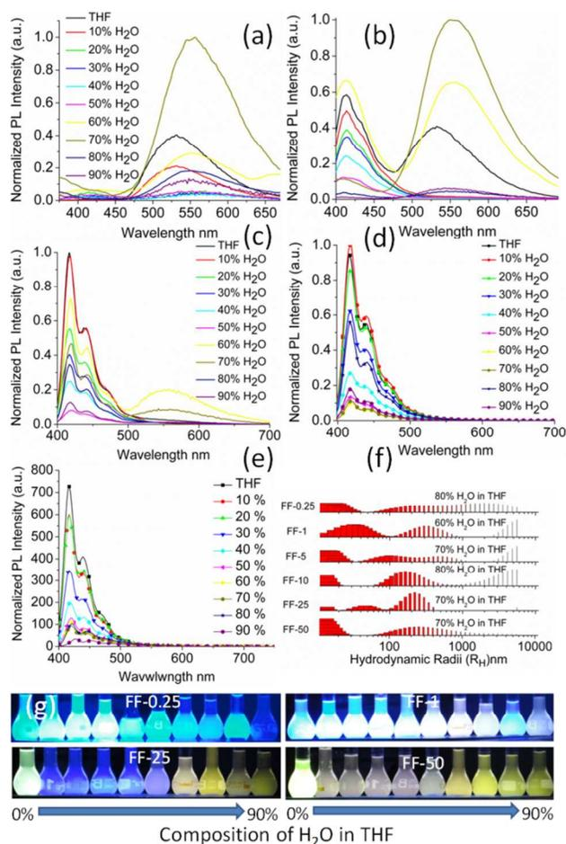
Figure 2. PL spectra of (a) FF-50, (b) FF-25, (c) FF-1, (d) FF-0.25, (e) poly 9,9-Dihexylfluorene-2,7-diyl (P9,9-DHF) in THF-water mixtures; (f) DLS traces of copolymers and (g) photograph of copolymer upon irradiation with  $\sim 360$  nm in different THF-water mixtures.
