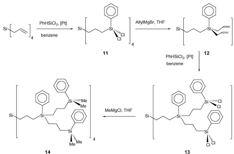
**Scheme 3** Synthesis of the carbosilane dendrimers **11–14** containing phenyl-Si groups at the branching points and in the periphery.
