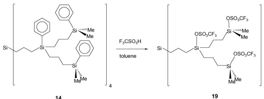
**Scheme 6** Acidolytic cleavage of the phenyl-Si groups at the branching points and in the periphery of **14** giving the highly reactive triflate-Si derivative **19**.
