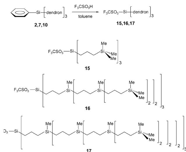
**Scheme 4** Acidolytic cleavage of the core phenyl-Si groups in PhSiR<sub>3</sub> dendrimers with triflic acid giving triflate-Si core units.
