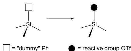
The strategy is thus straightforward: introducing phenyl groups at different points of a carbosilane dendrimer as “dummy” functions which can be selectively converted to highly reactive triflate groups which in turn are readily substituted by anionic nucleophiles. To which degree dummy functions in
