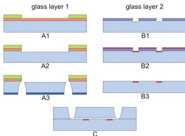
**Fig. 3** Schematic diagram of the fabrication process. Glass layer 1 is firstly sputtered with Cr and Au, which is subsequently coated with a resist. After several lithography steps (A1), the microchannel is made by isotropically etching (A2). Access holes were powder blasted (A3). On glass layer 2 first a lithography step is done (B1). Subsequently platinum is sputtered (B2) and the electrodes are created by lift-off (B3). Bonding of the two glass wafers (C) creates the chip.
