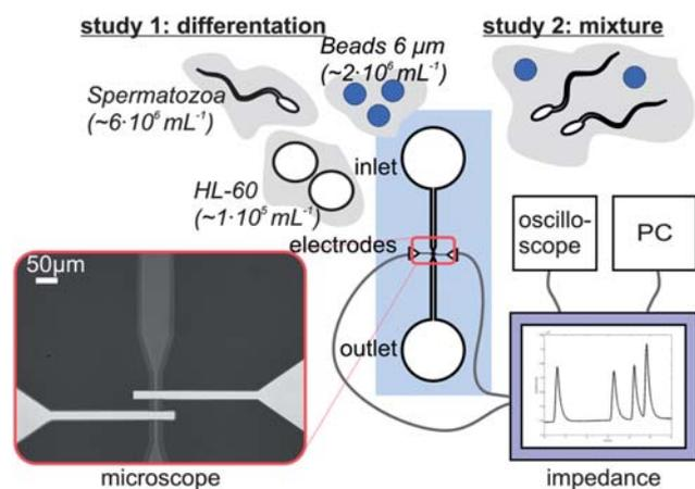
**Fig. 2** A schematic picture of the measurement set-up. The microfluidic chip is connected to the home-made impedance analyzer, which is connected to a PC and an oscilloscope. Visual inspection of the set-up is possible using an inverted microscope. Different samples are used for the two studies.
