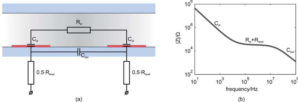
**Fig. 1** (a) The simplified equivalent circuit model of the microfluidic device without a particle or cell in the channel. The interface between the two planar electrodes and the electrolyte is represented by the double layer capacitance ( $C_{dl}$ ).  $R_{el}$  is the electrolyte resistance,  $R_{lead}$  the lead resistance and  $C_{par}$  is the parasitic capacitance. (b) Typical frequency response of the real electrical impedance of the equivalent circuit model.
