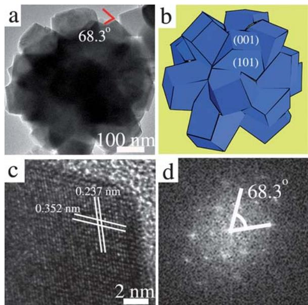
**Fig. 2** (a) TEM image of the flower-like  $\text{TiO}_2$  nanostructures. (b) Schematic diagram of the flower-like  $\text{TiO}_2$  nanostructures. (c) HRTEM image of a truncated tetragonal pyramidal  $\text{TiO}_2$  nanocrystal. (d) The corresponding fast-Fourier transform (FFT) pattern.
