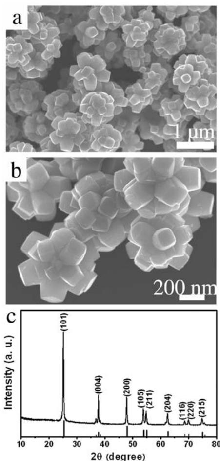
**Fig. 1** (a, b) FE-SEM images of the flower-like  $\text{TiO}_2$  nanostructures at low and high magnifications, respectively. (c) XRD pattern of the flower-like  $\text{TiO}_2$  nanostructures. Vertical bars indicate peak position and intensity of anatase  $\text{TiO}_2$  (JCPDS No. 21-1272).
