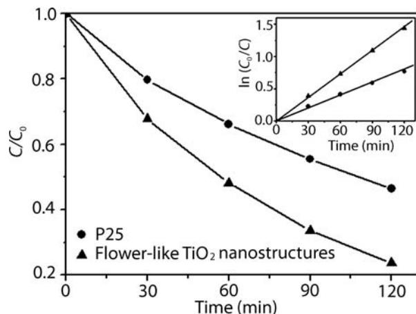
**Fig. 3** The variation of MB concentration by photoelectrocatalytic reaction with P25  $\text{TiO}_2$  powders and flower-like  $\text{TiO}_2$  nanostructures. The inset shows the pseudo-first-order kinetic rate plots for the photochemical degradation of MB.
