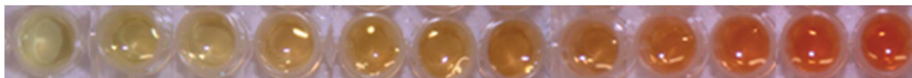
Fig. 5 Results of limit of detection testing of BZP HCl using the NQS colour test method performed in plastic micro-well plates. Amounts used are 0, 1, 2, 4, 5, 7, 9, 10, 20, 30, 40 and 50 \mu\text{g} , respectively.
