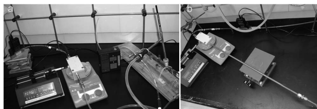
Fig. 2 Vapour-generation system, comprising mass flow controller, vaporisation unit and syringe pump. Image a shows the generator connected to a 1.5 L gas sampling tube into which the dynamic SPME sampler is inserted, while image (b) shows the generator connected to a glass funnel.
