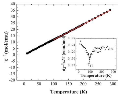
**Fig. 6** Inverse magnetic susceptibility data  $\chi^{-1}$  vs.  $T$  and  $d\chi^{-1}/dT$  vs.  $T$  (inset) for  $\text{Ba}_2\text{GdMoO}_6$ , evidencing the structural transition from tetragonal to triclinic symmetry below 100 K.
