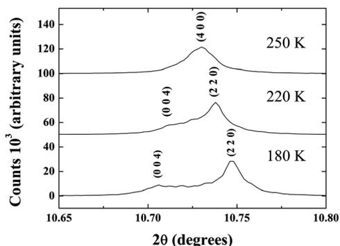
**Fig. 2** A selected area of the synchrotron X-ray diffraction pattern of  $\text{Ba}_2\text{GdMoO}_6$  showing the [400] structural peak at 250 K (top). There is clear evidence of peak splitting at the cubic to tetragonal phase transition displayed here for  $T = 220$  K (middle) and 180 K (bottom). This peak splitting increases upon reducing the temperature.
