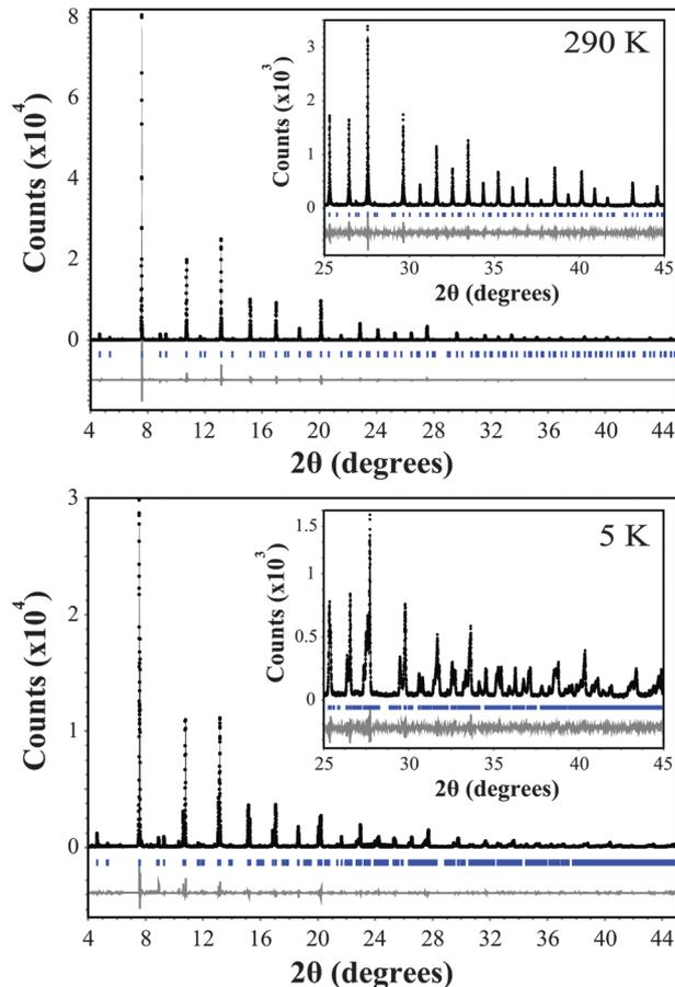
**Fig. 1** Rietveld refinement of the synchrotron X-ray diffraction data for  $\text{Ba}_2\text{GdMoO}_6$ . The black line represents the actual data, the black circles represent the calculated pattern and the trace below is the difference between calculated and collected data. A region between 6.65 and 7.45  $2\theta$  (degrees) is excluded due to a peak associated with a small amount of unknown impurity.
