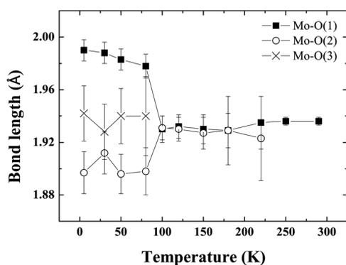
**Fig. 5** The thermal evolution of the Mo–O bond lengths in  $\text{Ba}_2\text{GdMoO}_6$ . There is no evidence of the Jahn–Teller distortion previously reported for  $\text{Ba}_2\text{LnMoO}_6$  ( $\text{Ln} = \text{Nd}, \text{Sm}$ ).
