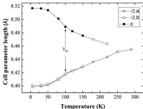
**Fig. 4** Evolution of the cell parameters with temperature evidencing a structural transition to triclinic symmetry below 100 K ( $T_{\text{Tri}}$ ); a and b have been multiplied by  $\sqrt{2}$  for ease of comparison.
