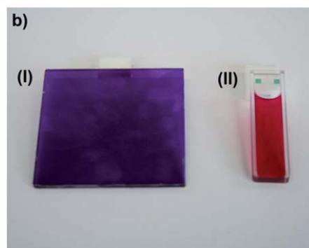
Fig. 3 Absorption spectra (a) and photographs (b) of cyanidin chloride in PLA (I) ( $c = 0.213$  mg g<sup>-1</sup>,  $T = 20$  °C and  $d = 2$  mm) and in dodecyl gallate (II) ( $c = 0.213$  mg g<sup>-1</sup>,  $T = 100$  °C and  $d = 1$  mm for the spectrum and 2 mm for the photograph).
