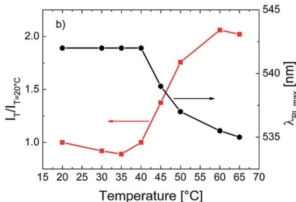
**Fig. 3** (a) The effect of temperature on the fluorescence characteristics of **P-2** in PBS ( $0.1 \text{ g L}^{-1}$ ). The excitation wavelength was 435 nm. (b) The correlation between  $\lambda_{\text{PL,max}}^{\text{PL}}$ , the relative emission intensity ( $I_T/I_{T=20^\circ\text{C}}$ ), and the temperature of the solution. Data are taken from the spectra in (a).
