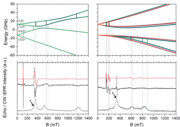
**Fig. 3** Top: Zeeman diagrams for the  $S = 3/2$  ground state and X-band EPR transitions calculated for  $\theta = 8^\circ$  (left) and  $90^\circ$  (right; different colours represent the four molecular orientations, see text). Bottom: experimental (black) and simulated (red) CW, and FSED (grey) spectra at 5 K. [The peak at 330 mT, marked \*, is intrinsic to the resonator.]
