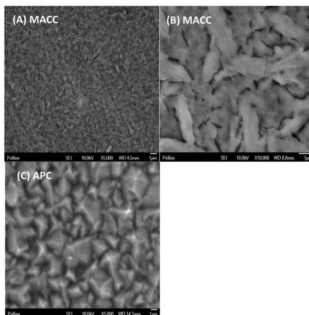
Fig. 3 Displays SEM micrographs of about 5 μm thick Mg resulting from galvanostatic plating of Mg onto a Pt working electrode at 1 mA cm<sup>-2</sup>. 0.25 M MACC 2 : 1 solution in DME is shown at lower and higher magnification in 3A and 3B, respectively. 3C results from 0.25 M APC 2 : 1 under the same conditions.
