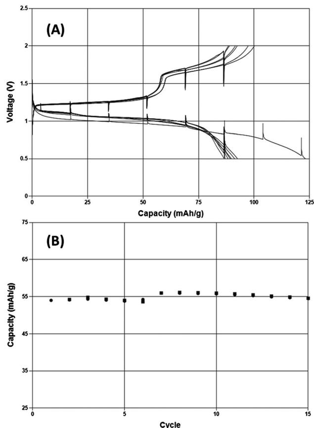
Fig. 4 Galvanostatic cycling of  $\text{Mo}_6\text{S}_8$  in 0.25 M MACC 3 : 2 in DME taken at  $C/15$  for several cycles, shown as a voltage profile in (A) and followed by  $C/2$  for an additional 15 cycles depicted as charge and discharge capacity vs. cycle number (B). Mg serves as the negative electrode.
