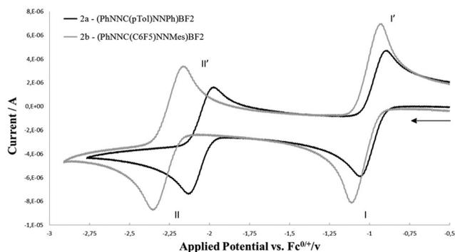
Fig. 1 Cyclic voltammetry of **2a** and **2b** (1.5 mM solution in THF, 0.1 M [Bu<sub>4</sub>N][PF<sub>6</sub>]) recorded at 100 mV s<sup>-1</sup>.
