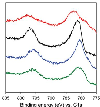
**Fig. 3** X-ray photoelectron spectroscopy (XPS) spectra of CoSal<sup>tBu,R<sub>2</sub></sup> compounds showing the Co 2p<sub>3/2</sub> and 2p<sub>1/2</sub> binding energies (red: R<sub>2</sub> = NO<sub>2</sub>; black: R<sub>2</sub> = *t*Bu; blue: R<sub>2</sub> = OMe; green: R<sub>2</sub> = NMe<sub>2</sub>). Full spectra shown in Fig. S2.†
