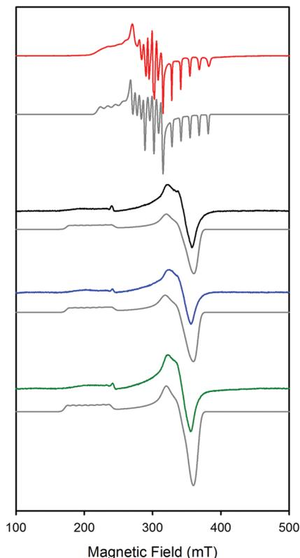
**Fig. 4** X-band EPR spectra of CoSal<sup>tBu,R2</sup>. Red: R<sub>2</sub> = NO<sub>2</sub>,  $\nu = 9.384$  GHz; black: R<sub>2</sub> = tBu,  $\nu = 9.383$  GHz; blue: R<sub>2</sub> = OMe,  $\nu = 9.383$  GHz; green: R<sub>2</sub> = NMe<sub>2</sub>,  $\nu = 9.385$  GHz. Grey spectra are respective simulations. Conditions: power = 2.0 mW; modulation frequency = 100 kHz; modulation amplitude = 0.4 mT;  $T = 20$  K.
