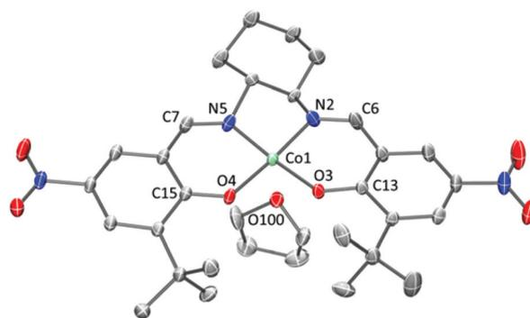
**Fig. 1** POV-ray representation (50% probability) of CoSal<sup>tBu,NO2</sup>·THF, excluding hydrogen atoms. Selected interatomic distances (Å) and angles (°): Co(1)–O(4), 1.901; Co(1)–O(3), 1.895; Co(1)–N(5), 1.876; Co(1)–N(2), 1.874; N(5)–C(7), 1.292; N(2)–C(6), 1.288; O(4)–C(15), 1.296; O(3)–C(13), 1.291; Co(1)–O(100), 2.211; O(3)–Co(1)–O(4), 86.9(4); O(4)–Co(1)–N(5), 93.5(7); O(3)–Co(1)–N(2), 93.4(8); N(2)–Co(1)–N(5), 85.2(7).
