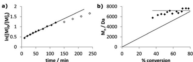
**Fig. 6** Plots of (a)  $\ln([M]_0/[M]_t)$  vs. time and (b) molecular weight vs. conversion for bulk styrene polymerisation at 120 °C using CoSal<sup>tBu,tBu</sup> and AIBN. Monomer : catalyst : initiator ratio of 100 : 1 : 0.6 used. Solid data points in (a) used to calculate least-squares fit. Solid line in (b) represents  $M_{n,\text{th}}$ , while dashed line indicates ‘top-out’ molecular weight.
