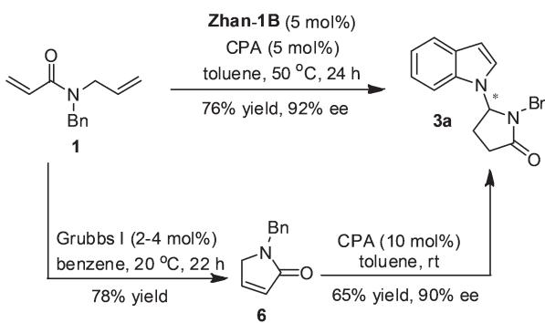
**Scheme 3** Comparison between cascade reaction and stepwise reaction.
