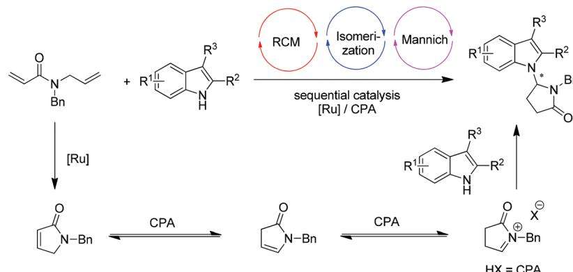
**Scheme 1** Ring-closing metathesis/isomerization/Mannich reaction sequence.**Table 1** Screening of chiral phosphoric acids
