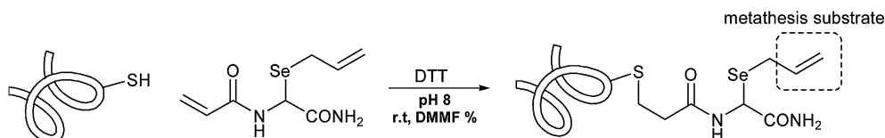
Scheme 6 Protein surface modification by reaction with Seac-acrylamide.
