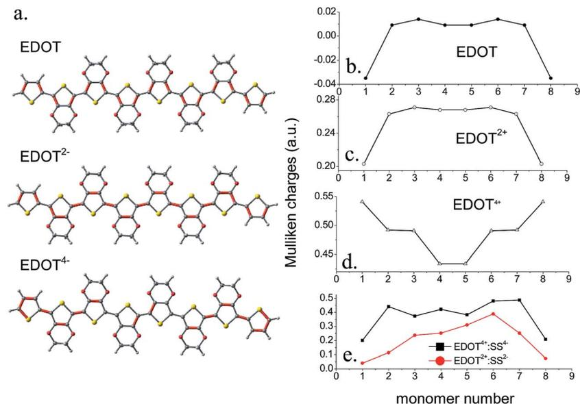
Fig. 5 (a) Nature of bond alternation in EDOT, EDOT<sup>2+</sup> and EDOT<sup>4+</sup>. The red bonds are aromatic double bonds (1.38–1.39 Å for C=C and 1.70 Å for C=S). (b) Mulliken charges for EDOT. (c) Mulliken charges for EDOT<sup>2+</sup>. (d) Mulliken charges for EDOT<sup>4+</sup>. (e) Mulliken charges for EDOT<sup>2+</sup>–SS<sup>2-</sup> and EDOT<sup>4+</sup>–SS<sup>4-</sup>.
