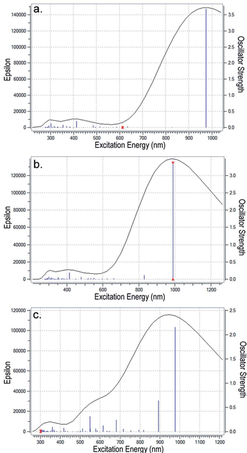
Fig. 7 The UV-vis spectra for (a) PEDOT<sup>2+</sup> (without PSS<sup>2-</sup> counterion); (b) PEDOT<sup>2+</sup> slightly bent to interact with the dianion; and (c) PEDOT<sup>4+</sup> with more bending when it interacts with the tetracation.
