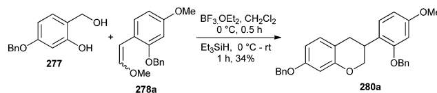
Scheme 59 [4 + 2] Cycloaddition reaction of substituted phenol with enol ether 278a.
