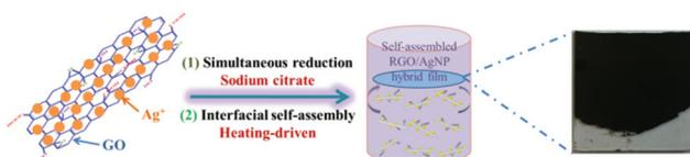
Fig. 2 Schematic model for fabricating RGO/AgNP hybrid film.
