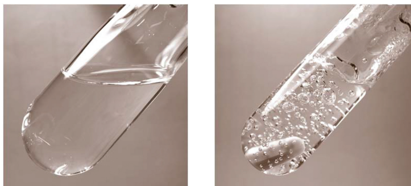
Fig. 1 Photographs of a \text{MgF}_2 sol (left) and \text{MgF}_2 gel with air bubbles (right).
