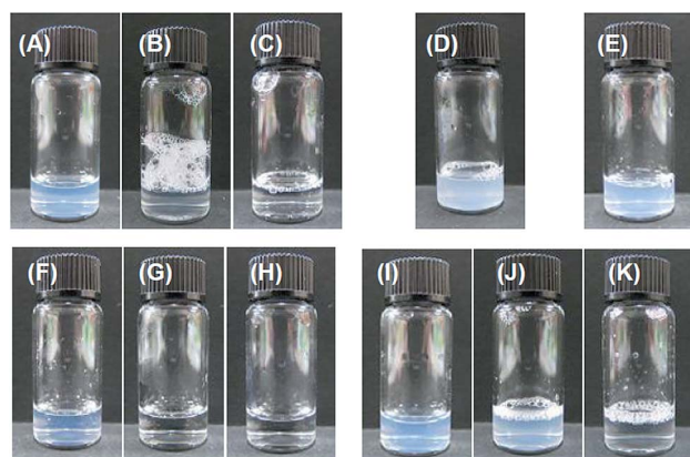
Fig. 2 Photographic images of aqueous solutions of the DMPC liposomes both (A) before and after the addition of (B) 10 equiv. and (C) 20 equiv. of DMe- \beta -CDx. Photographic images of the DMPC liposomes after the addition of (D) 20 equiv. of TMe- \beta -CDx and (E) 20 equiv. of \gamma -CDx. Photographic images of the DLPC liposomes (F) before and after the addition of (G) 10 equiv. and (H) 20 equiv. of DMe- \beta -CDx. Photographic images of the DPPC liposomes (I) before and after the addition of (J) 10 equiv. and (K) 20 equiv. of DMe- \beta -CDx ([lipids] = 1.0 mM).
