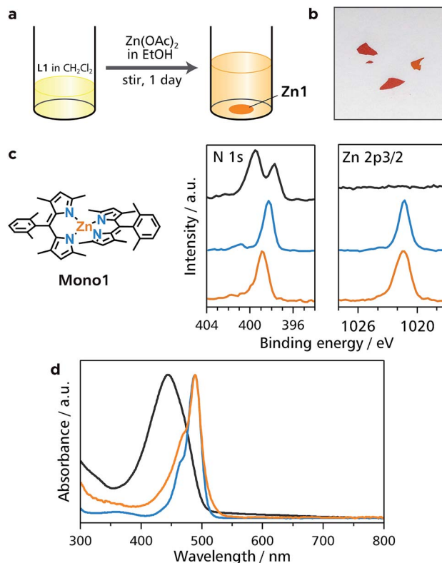
Fig. 2 Single-phase synthesis and characterization of Zn1 . (a) Schematic illustration of the synthesis. (b) Photograph of powdery Zn1 . (c) Chemical structure of referential compound Mono1 , and XPS of L1 (black), Mono1 (blue), and Zn1 (orange) focusing on the N 1s and Zn 2p 3/2 regions. (d) UV/vis spectra of L1 (black), Mono1 (blue), and Zn1 (orange) in DMF.
