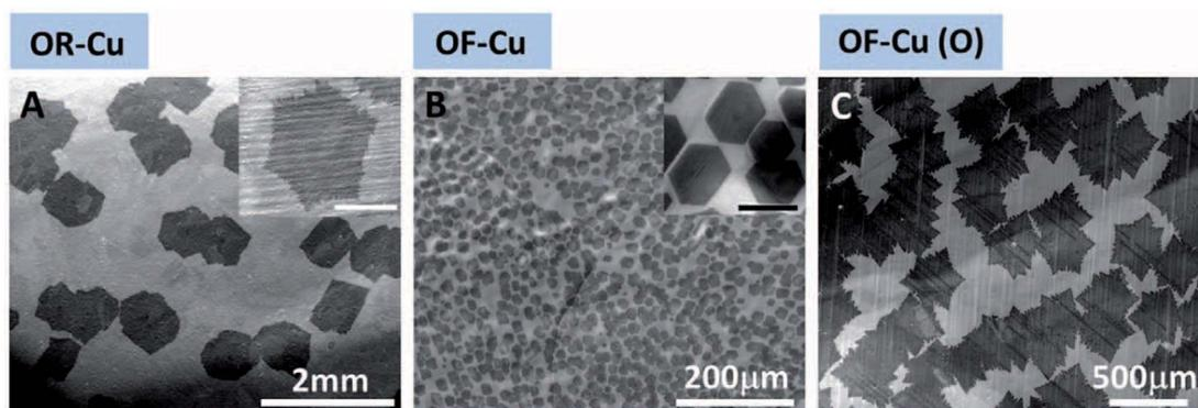
Fig. 3 The effect of O on graphene nucleation density and domain shapes on various types of Cu substrates. OR-Cu (A) represents low-purity copper substrates, OF-Cu (B) represents high-purity copper substrates, and OF-Cu (O) (C) represents high-purity copper substrates exposed to oxygen before the CVD growth of graphene. Reprinted from ref. 47 by permission of American Association for the Advancement of Science.
