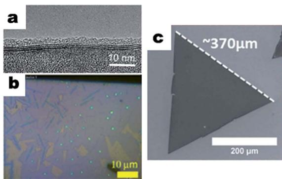
Fig. 5 (a) TEM image of CVD grown few layer MoS<sub>2</sub>, reprinted from ref. 73 by permission of John Wiley & Sons; (b) optical microscopy image of CVD synthesized single layer MoS<sub>2</sub>, reprinted from ref. 75 by permission of American Chemical Society; (c) SEM image of a CVD synthesized single crystal WS<sub>2</sub> nanosheet, reprinted from ref. 82 by permission of the Royal Society of Chemistry.
