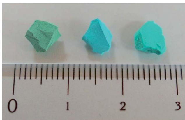
Fig. 2 Optical images showing representative samples of (left) the  $\text{Cu}(\text{OH})_2$ -polyacrylamide (PAAm) composite monolith, (center) after coordination replication to form the  $\text{Cu}_2(\text{bdc})_2(\text{MeOH})_2$  monolith, and (right) after PCP-to-PCP replication to form the  $\text{Cu}(\text{bdc})_2(\text{bpy})$  monolith.
