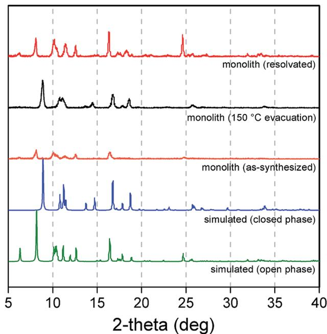
Fig. 6 Powder X-ray diffraction patterns simulated for the open (green) and closed (blue) forms of  $\text{Cu}_2(\text{bdc})_2(\text{bpy})$ , and experimental patterns for an as-synthesized sample of a  $\text{Cu}_2(\text{bdc})_2(\text{bpy})$  monolith (orange), after evacuation at  $150^\circ\text{C}$  (black), and resolution by immersion in methanol (red).
