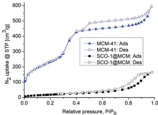
Fig. 4 N<sub>2</sub> sorption isotherms of MCM-41 and SCO@MCM samples; closed and open symbols refer to adsorption and desorption, respectively.
